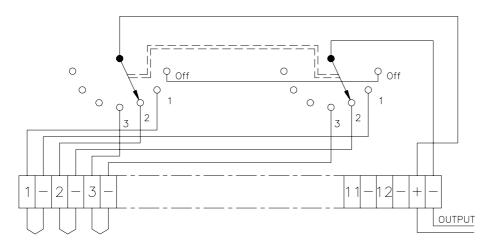
We recommend internal wiring of thermocouple material when temperature gradients are expected between terminals and switch contacts.
