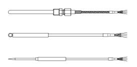
Resistance thermometer for direct immersion.
